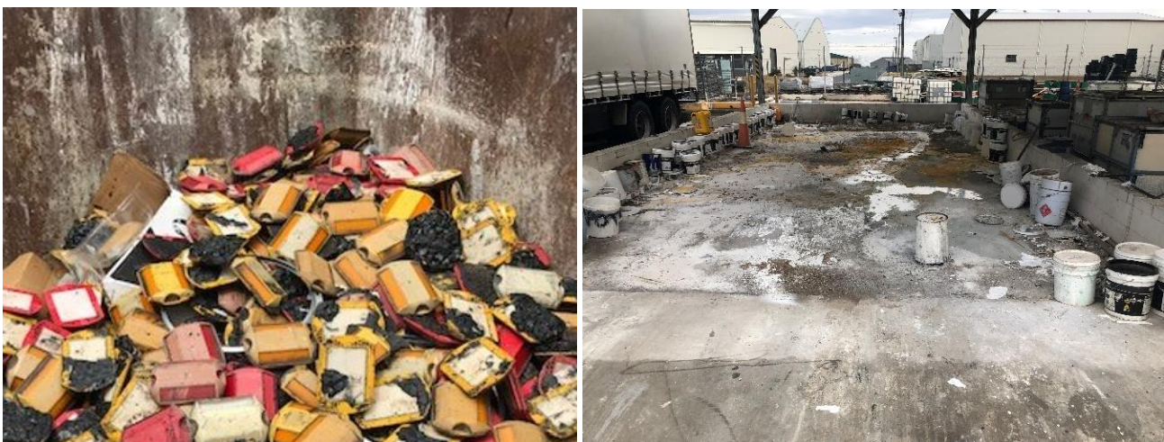
Exhibit 1.1. Photographs (provided by ARRB) of wastes being reviewed in this letter comprising 1) waste generated following RPM removal, and 2) typical wash bay where line marking equipment is washed into a sump and pumped to holding tank for disposal.
