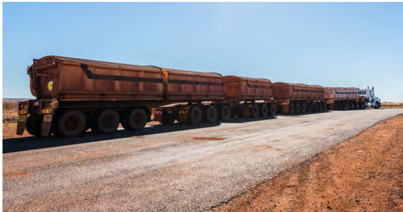
Australian road train on regional sprayed seal road. Image Source: Shutterstock 558511807
