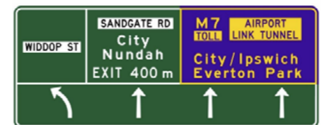
Examples of overhead lane designation style direction signs Image Source: TMR (2020)
