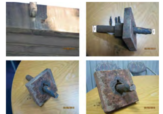
Broken sections of TSB on Bridge ID 7330 (Jun 2010 L2 inspection) Image Source: NACOE (2019)
