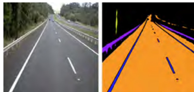
Attributes: road, line, metal barrier and tree (left: original image, right: recognition result) Image Source: NACOE (2019)
