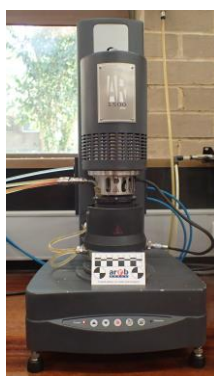
(h) DSR testing equipment
