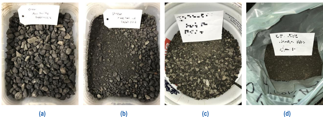
Figure 3.1: Photos of collected RAP samples, (a) contractor A coarse RAP, (b) contractor A fine RAP, (c) contractor B RAP, (d) contractor C RAP
