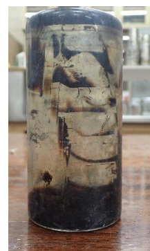
(f) Binder layer scraped out
