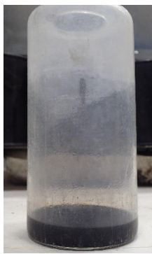
(a) Binder solution in RTFO bottle
