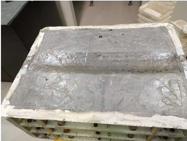
Figure G.3: Sealed surface after wheel tracking
