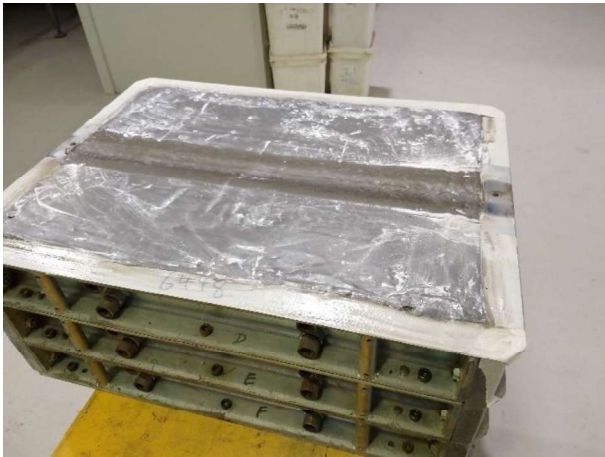
Figure G.15: Sealed surface after wheel tracking
