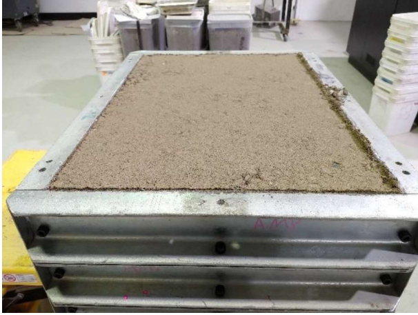
Figure G.1: Surface after compaction
