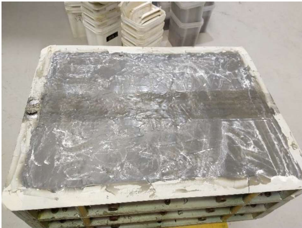
Figure G.9: Sealed surface after wheel tracking
