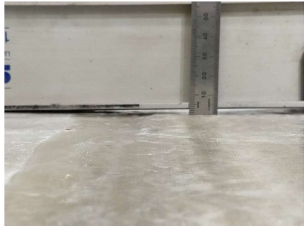
Figure G.16: Rut depth after 40 000 cycles
