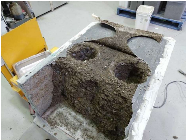
Figure G.11: Preparation for sand replacement
