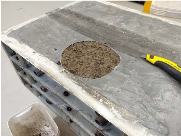
Figure G.5: Preparation for sand replacement
