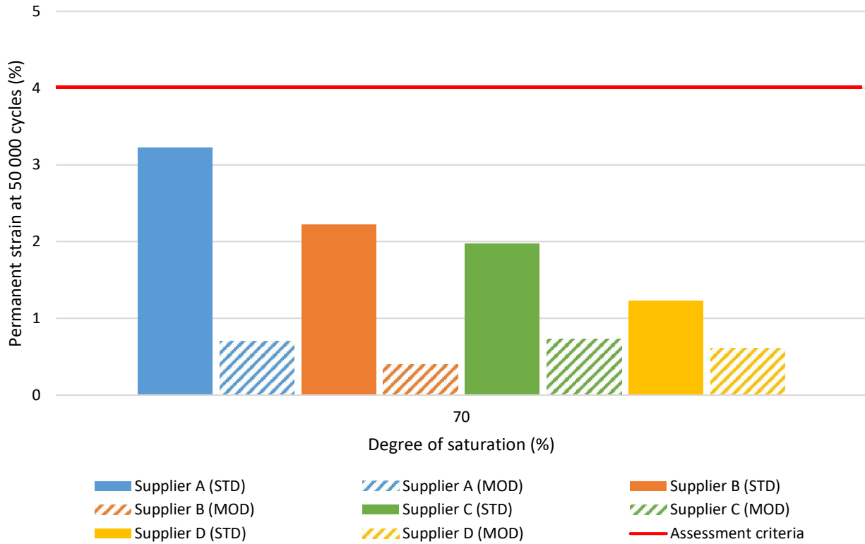
Figure 3.19: RM001 RLT permanent strain testing results at 50 000 cycles and 70% DOS
