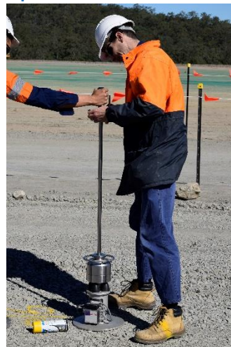
Spot test: Prima Light weight deflectometer (LWD)
