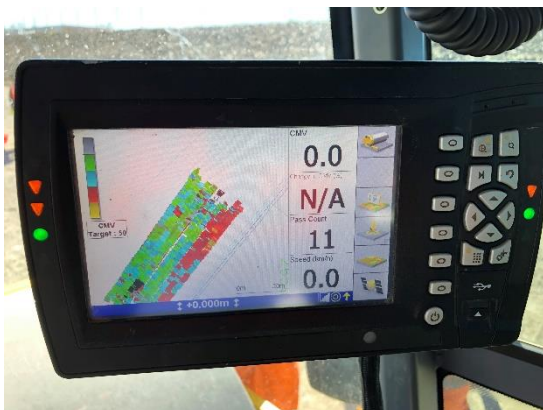
On-board display for real-time feedback to roller operator
