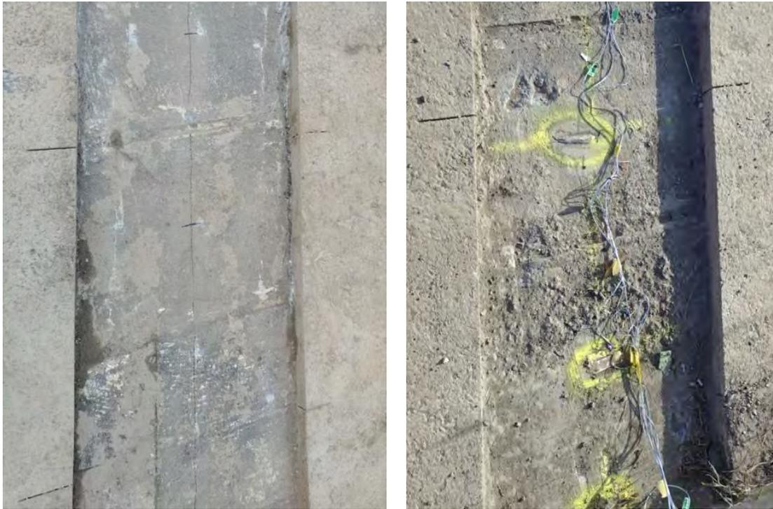
Notes: View of the exposed DU after DWS milling (left), and application of SGs on the top of each DU in mid width (right).
