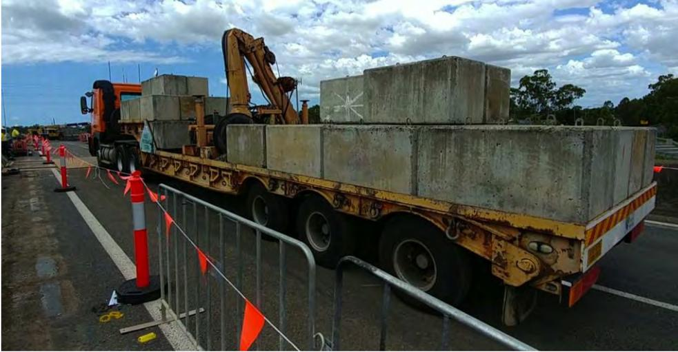
Figure D 2: View of the RMS truck loaded with 82.5 t moving along the northern path
