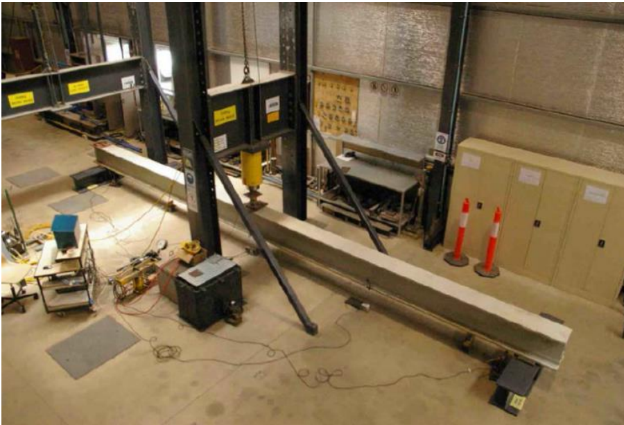
Figure 4.2: Typical setup for bending tests
