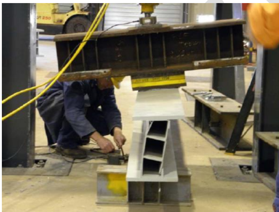
Figure 7.1: Failure of WCFT S2 girder in ultimate shear test
