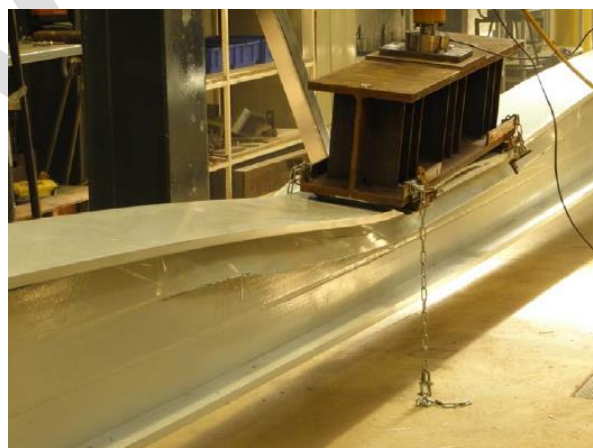
Failure of S2 girder in bending
