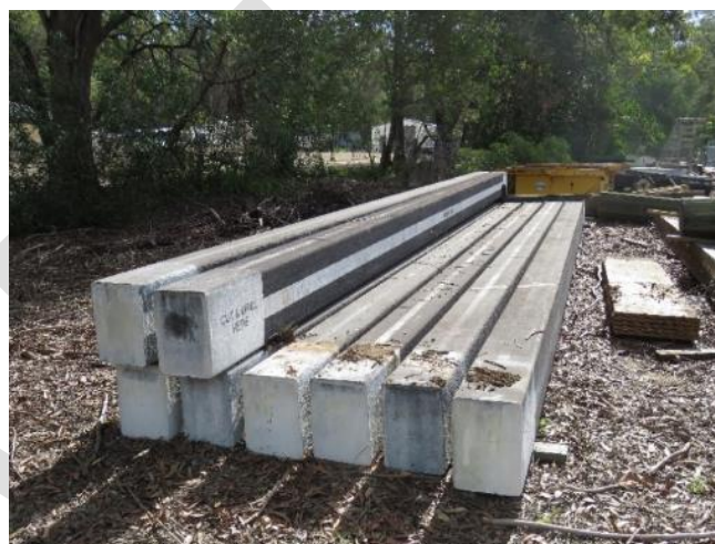
Girders type LOC400 at Nerang
