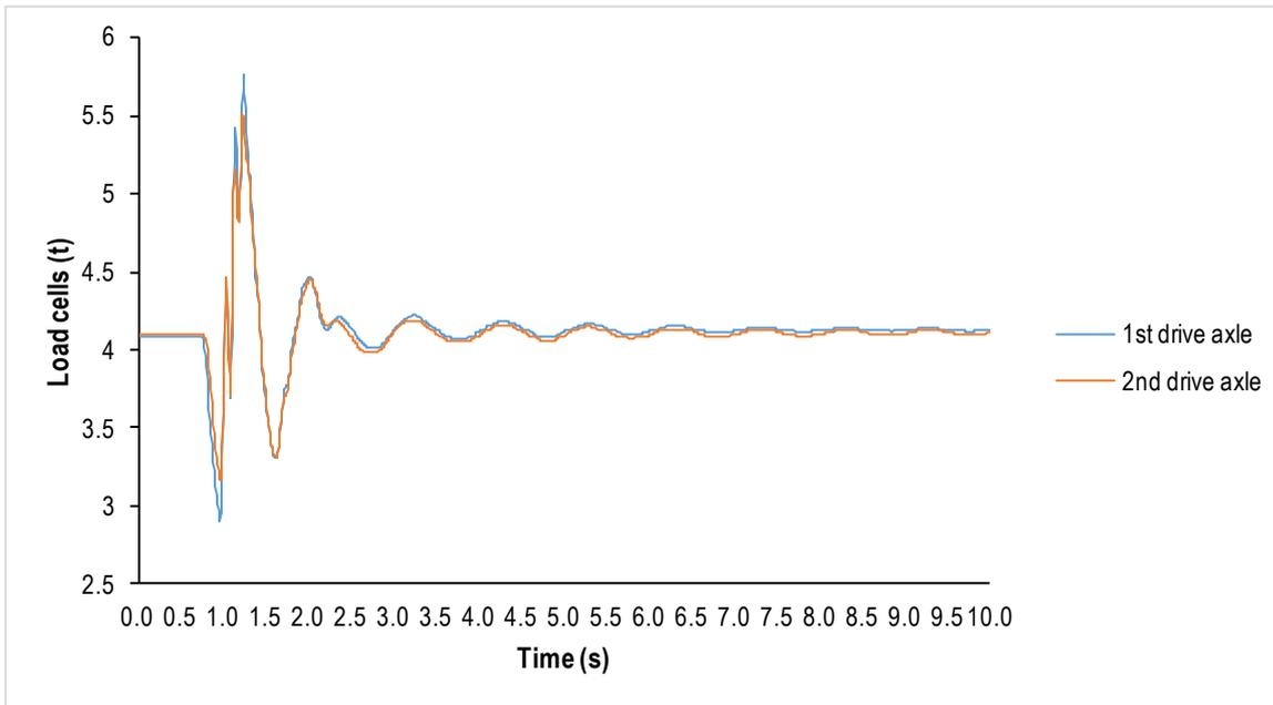
Figure C 26: Reference system (linear displacement) data trace from RFSA – HD shock absorbers
