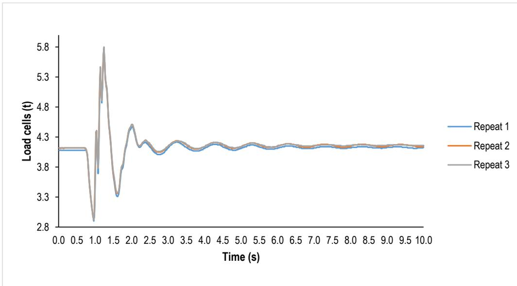
Figure C 24: Reference system (linear displacement) data trace from RFSA – HD shock absorbers
