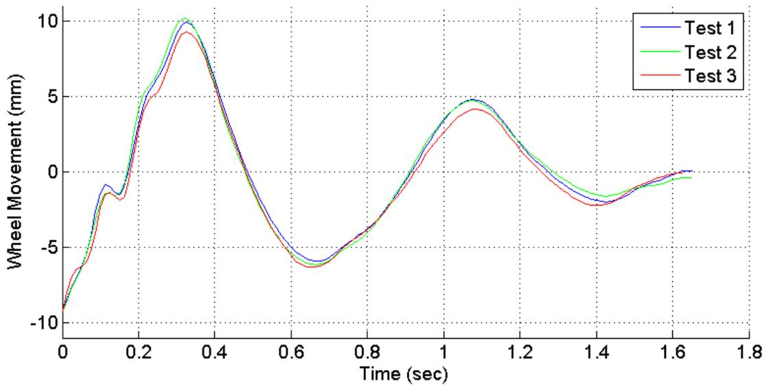
Figure C 37: Reference system data from DynaSsess test method with one shock absorber removed
