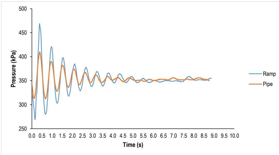
Figure C 13: Comparison of pipe and ramp tests using LDTs (LOW shocks – fully laden)
