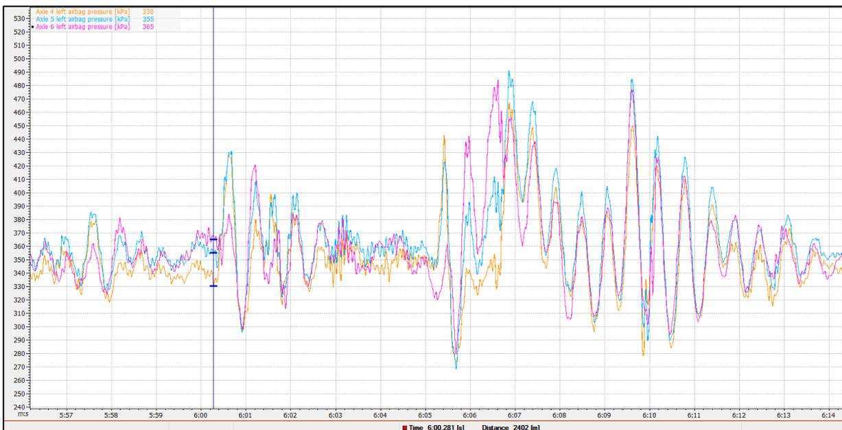
The data shown in Figure 7.2 and Figure 7.4 is for a period of 18 seconds, during which the vehicle travelling at 53 km/h crosses the four bridge joints and a repaired section of road as shown in Figure 7.5. The total bridge span was 50 m, with approximately 16.5 m between each joint. At the
