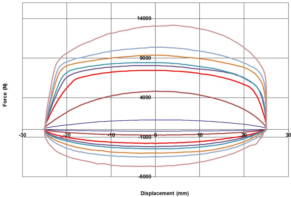
Figure B 15: Force vs displacement test results for a low damping shock absorber
