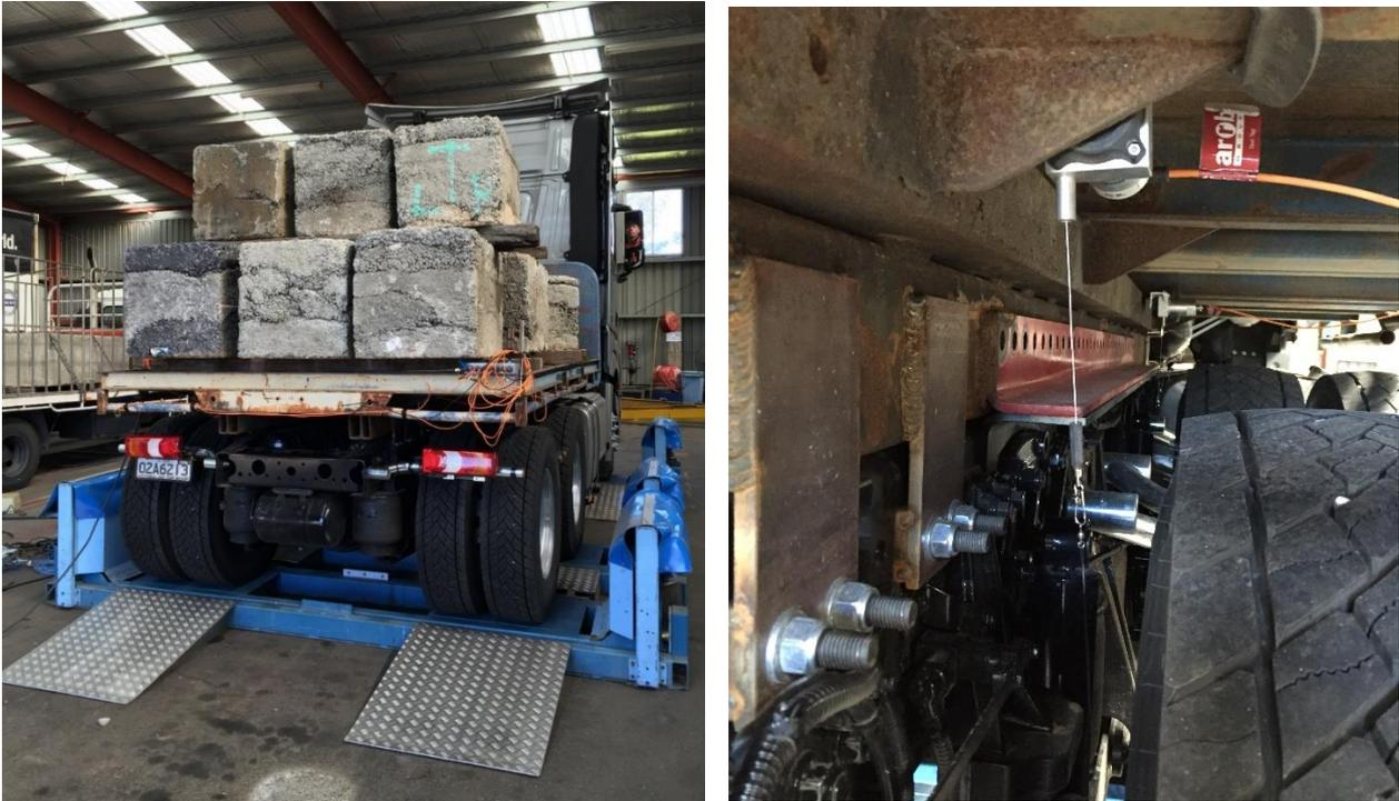
Figure 6.11 shows the DynaSsess system fitted to the rear axle of the 4x2 rigid truck. The system comprises three main components: the measurement device fitted to the hub and shown in the left photograph, the excitation device (ramps) shown in the right photograph, and the analysis software (not shown).
