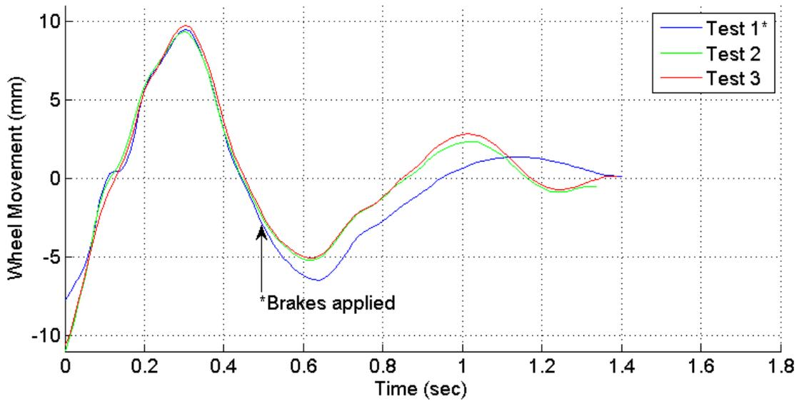
Figure C 34: FormulaSpec data from DynaSsess test method with all shock absorbers in place (flat road)
