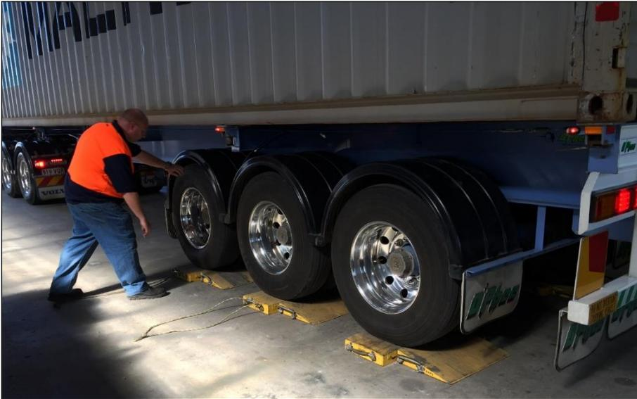
The vehicle should be travelling at 5 km/h when it falls off the step. This is not possible from a standing start, nor is it possible to have a 'run-up' as the disturbance created as the wheels mount the steps invalidates the response. For these reasons the VSB11 ramps are not considered to be a suitable excitation method for in-service testing. The variability in the test results (due to small differences in the position of the blocks between tests) confirms this finding.
