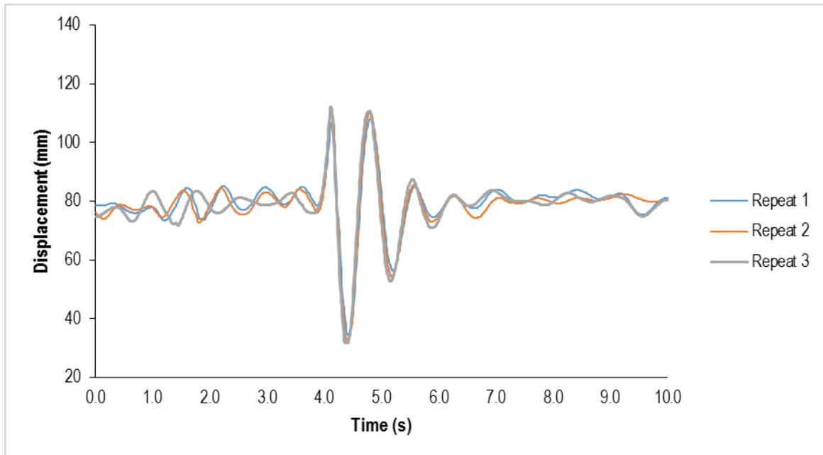
**C.3.6 Repeatability of VSB11 Tests: Fully Laden with all shock absorbers OFF**
