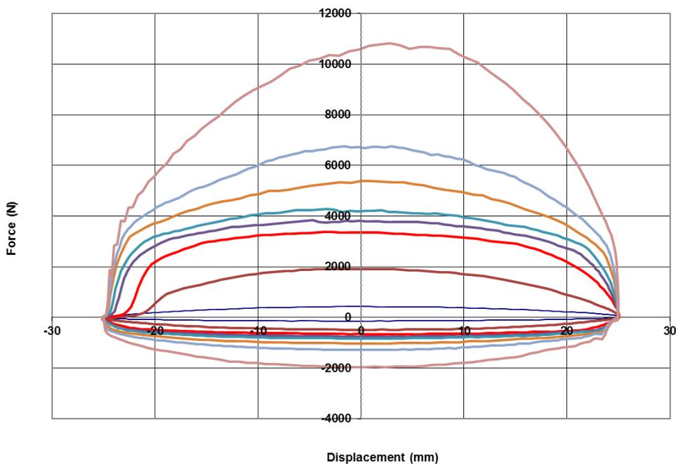
Figure B 16 shows a summary of the peak forces values for each shock absorber at four test speeds, for both the extension stroke and the compression stroke. The data points shown in the positive range of the y-axis represents the damping force in the extension stroke and compression stroke force is shown in the negative range. The four data points are four speeds at which the test were conducted: 0.13 m/s, 0.26 m/s, 0.39 m/s and 0.52 m/s.
