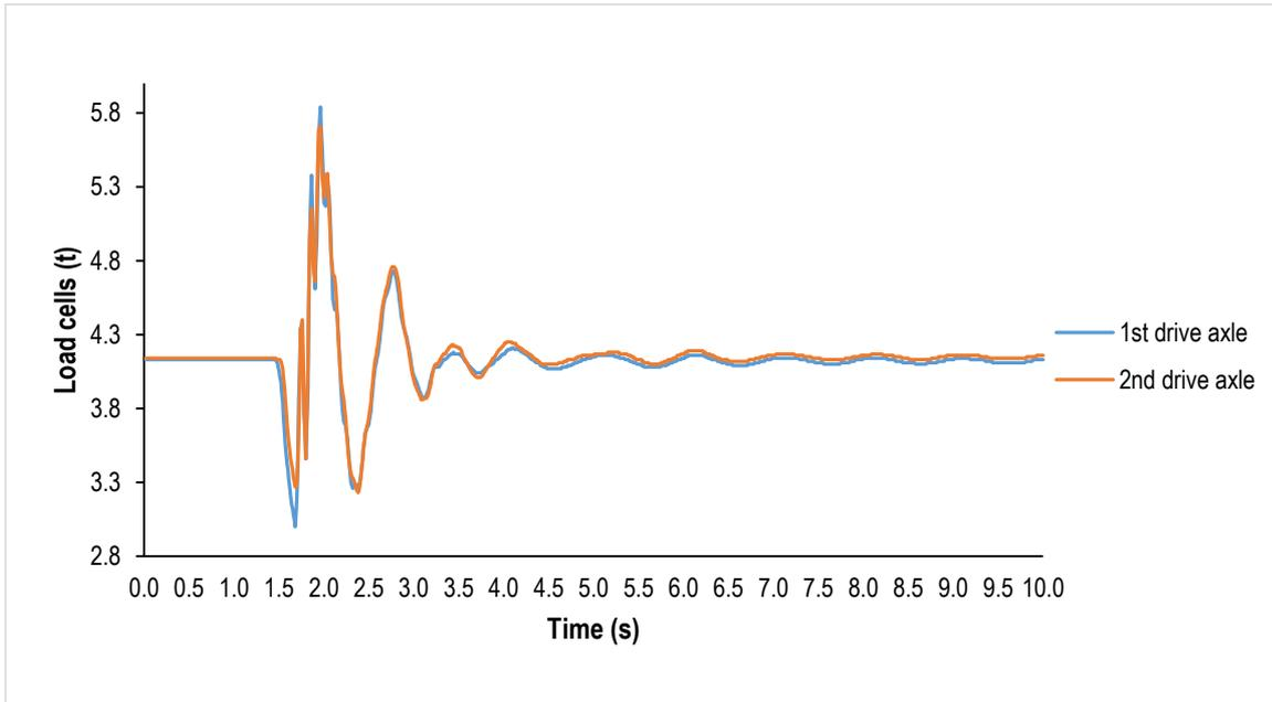
Figure C 28: Reference system (linear displacement) data trace from RFSA test – 1 shock absorber removed
