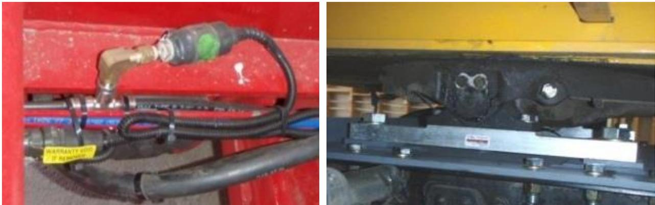
An EBS module is shown Figure 4.2. Such technology is common on trucks and prime movers and it is also becoming increasingly common on new trailers. This module is the basis for any electronic braking system; it can include sensors to record wheel speeds and air bag pressure and communicate with other devices via the controller area network (CAN). Data can be sent to the vehicle's telematics device and communicated via the mobile network or other wireless platforms.
