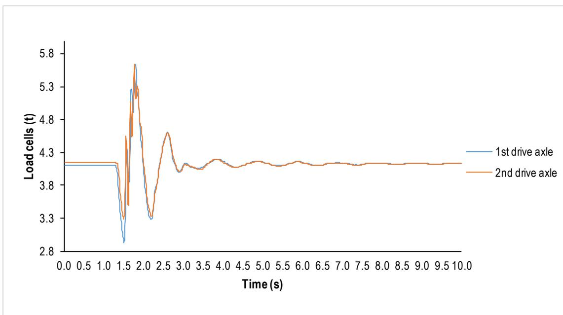
Figure C 30: Reference system (linear displacement) data trace from RFSA test – 1 shock absorber removed
