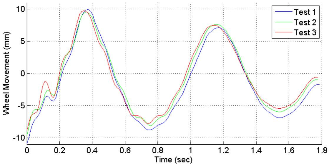
Figure C 39: Reference system data from DynaSsess test method with all shock absorbers removed
