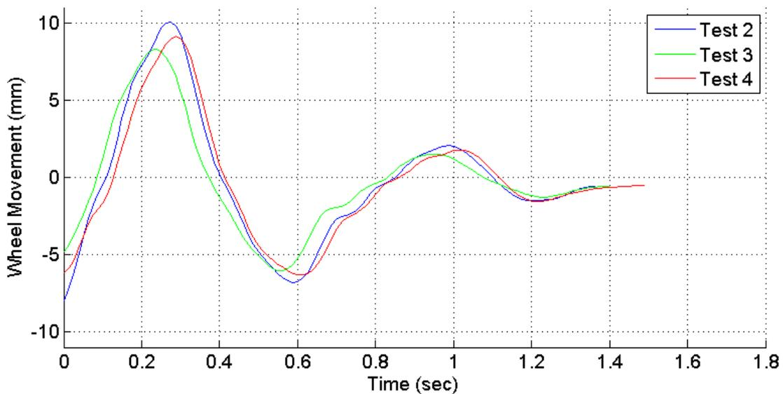
Table C 29: Reference system data from VSB11 ramp test method with all shock absorbers in place
