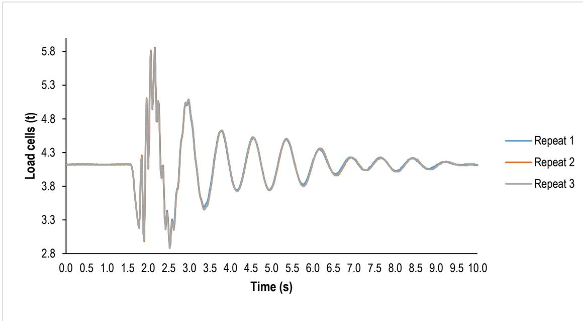
Figure C 32: Reference system (linear displacement) data trace from RFSA test – all shock absorbers removed
