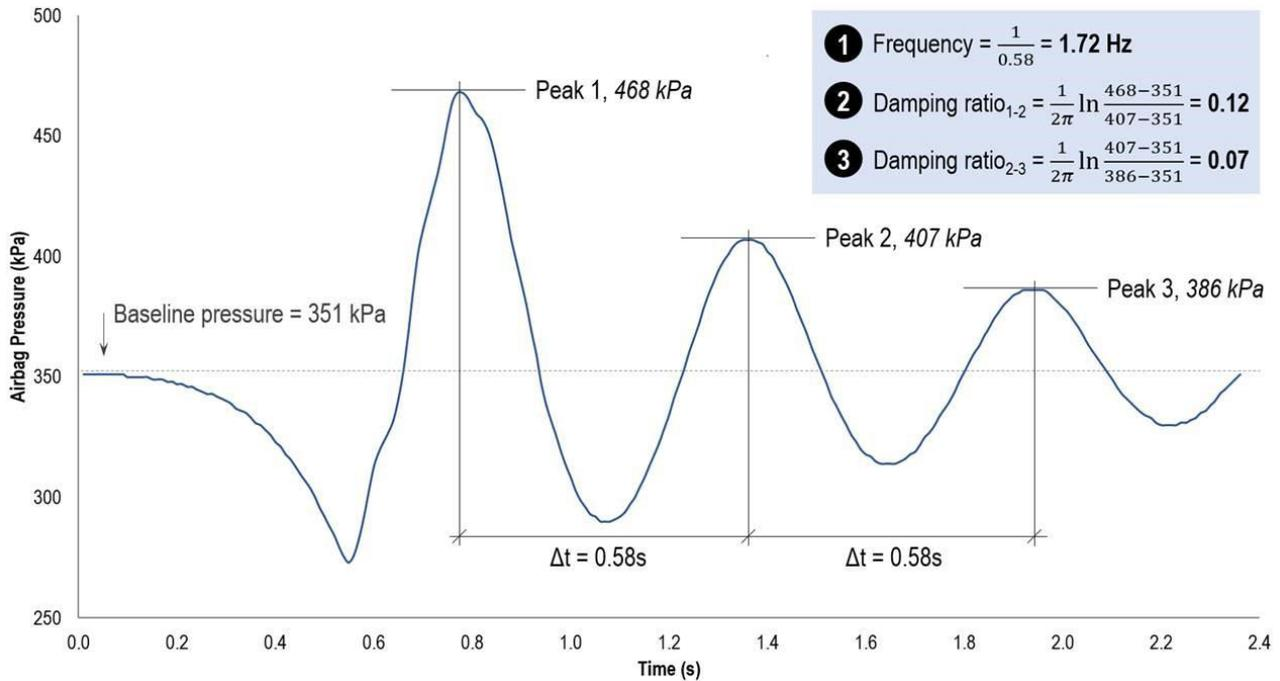
The other important step in analysing the data is to select the baseline value. It can be difficult to determine the true baseline value, particularly if the axles in the suspension group settle at a different positions following the test. Figure 9.4 shows the variation in damping depending on the baseline value selected. This example is based on data from Stage 1 testing; a damping ratio is 20% or 24% depending on which baseline value is used.
