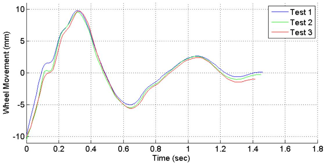
Figure C 35: Reference system data from DynaSsess test method with all shock absorbers in place
