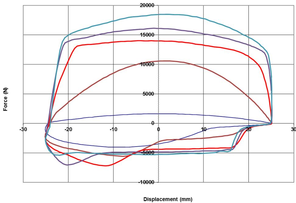
Figure B 14: Force vs displacement test results for a medium duty shock absorber
