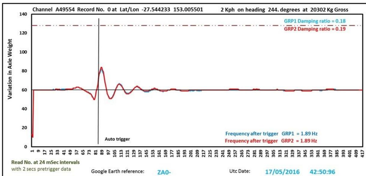
The processed data is 'zeroed' at a baseline value of 60 units. Therefore, this value of 60 represents zero vertical displacement between the axle and the body. It should be noted that air pressure transducers measure a voltage linearly proportional to the pressure, not displacement so this is not a direct measure of displacement. The damping ratio can be calculated by using subsequent peak values, as would be done by measuring the oscillation in vertical displacement, as per VSB11.
