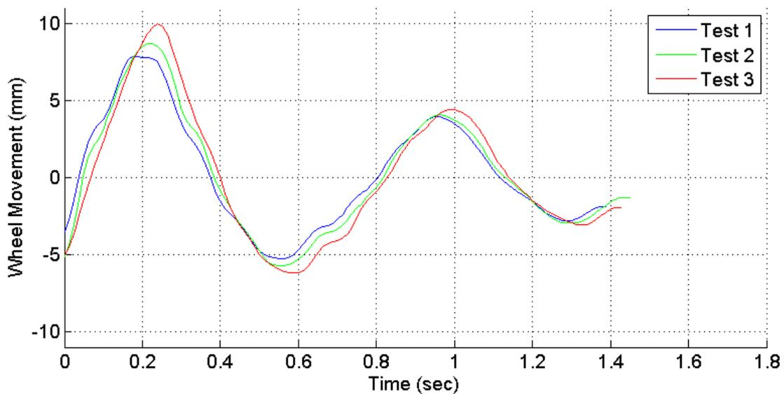
Figure C 41: Reference system data from VSB11 ramp test method with one shock absorber removed
