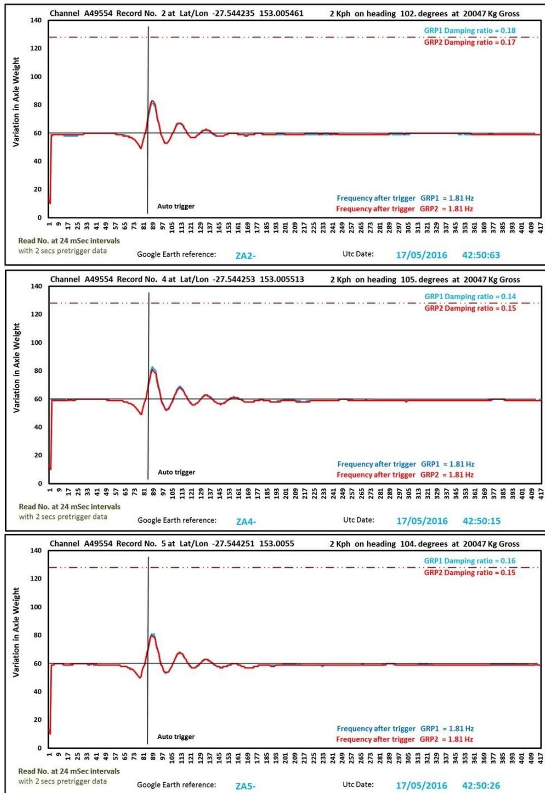
The frequency of each test is identical at 1.81 Hz, this is expected as the frequency of the suspension (which acts as a spring with constant stiffness) should not change. The damping ratio varies between left and ride sides and between tests. The damping ratio varies between 0.14 and 0.18, which is an increase of 28.5%.
