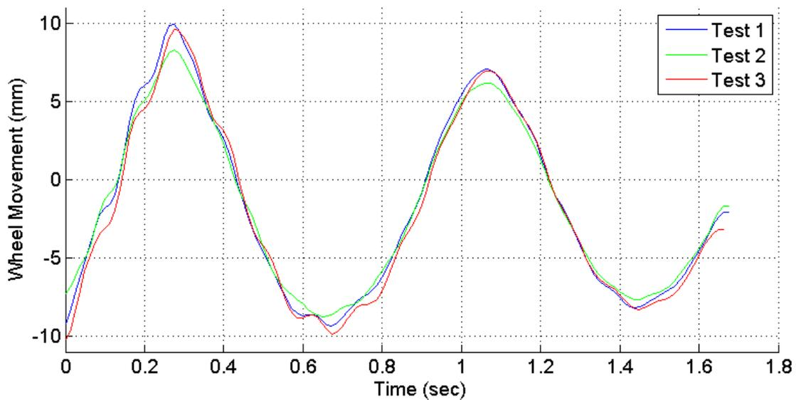
Figure C 43: Reference system data from VSB11 ramp test method with all shock absorbers removed
