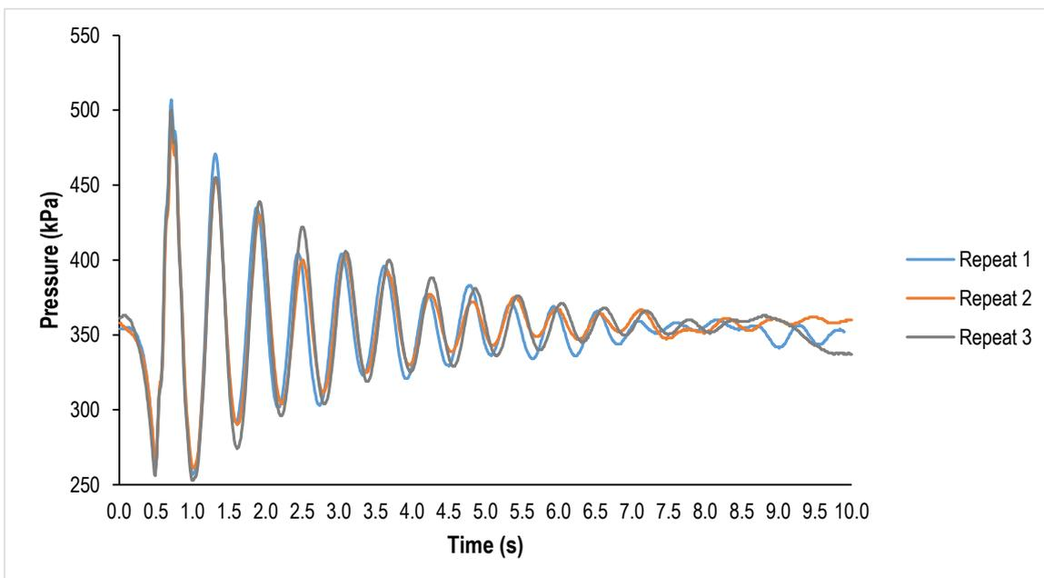
Figure C 11: Repeatability of pipe tests (NO shocks – fully laden)
