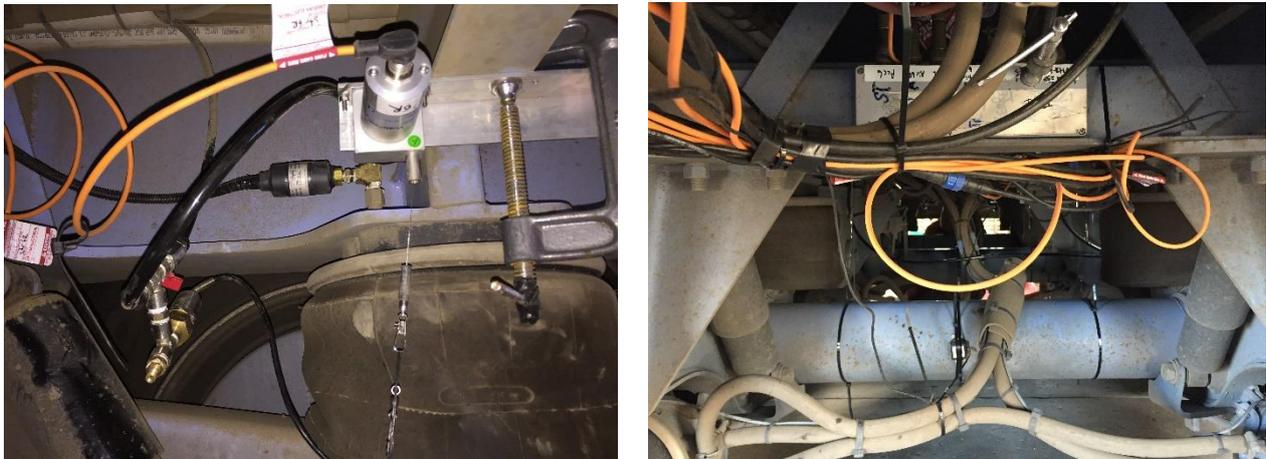
Figure 6.10 shows the RFSA rig with the fully laden 6x4 prime mover in position. The photograph on the left shows the LDT mounted between the underside of the tray and the rear axle. The excitation method for test program 2 was the VSB11 RFSA drop test, and the same method was used for both the test system and the reference system. The measurement methods were the load cell sensors permanently fitted to the RFSA system 2 and the LDTs fitted to each axle (reference system).
