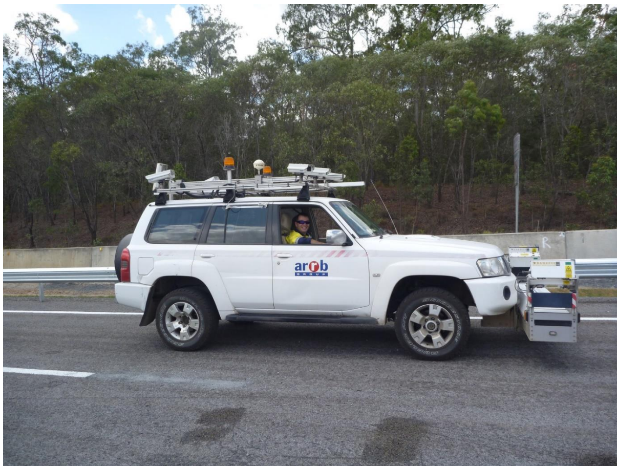
Figure 6.1: Measurement of rutting, roughness, texture and cracking
