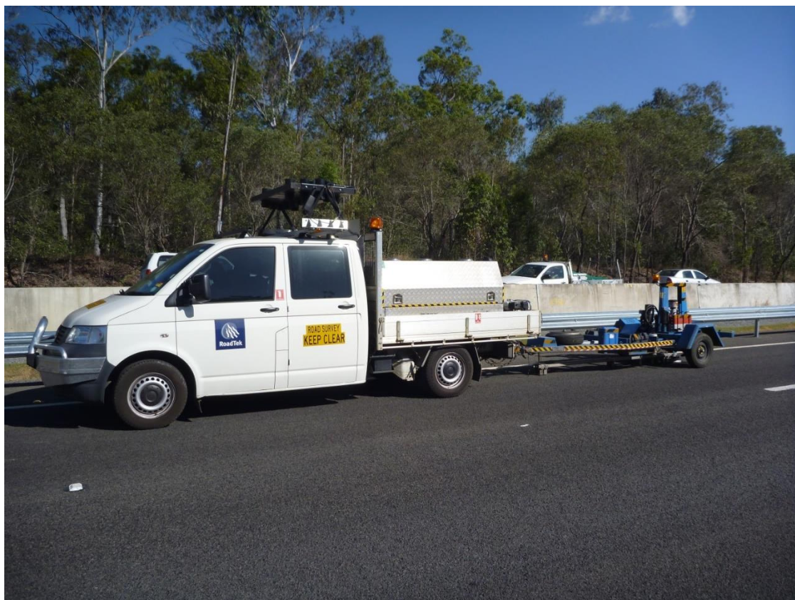
Figure 7.1: Falling weight deflectometer (FWD) assessing structural capacity of fast lane outside wheelpath
