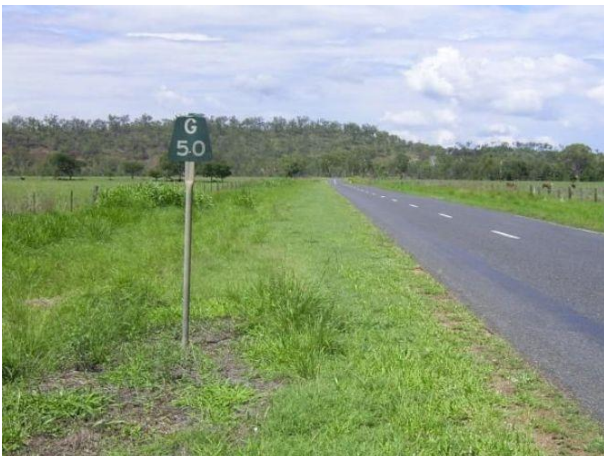
Figure 6.4: Wide clear zone (route sign with frangible pole)
