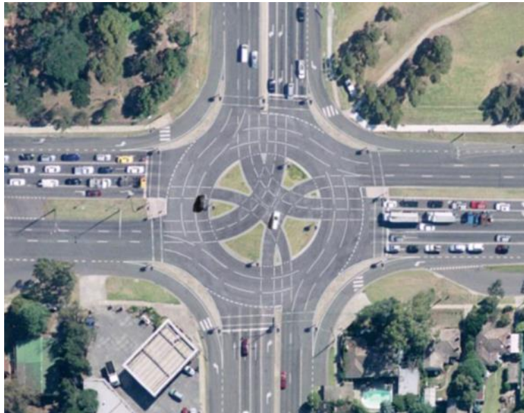
Figure 7.28: Example of a cut-through roundabout
