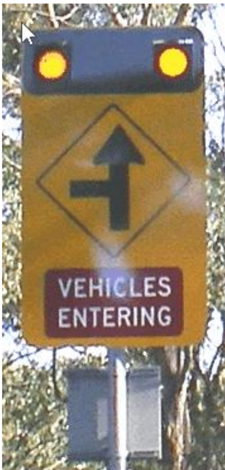
Figure 7.22: VAS on the approach to an intersection
