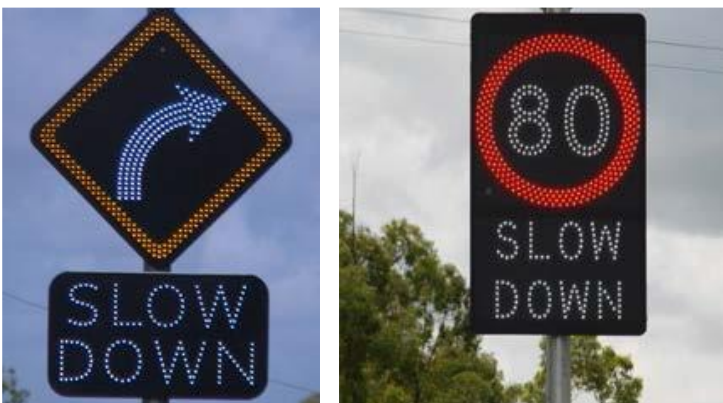
Figure 5.21: Examples of VAS used on approach to curve
