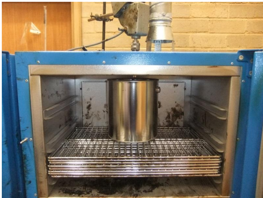
Figure 4.1: Laboratory blending of rubber-binder using oven and stirring equipment
