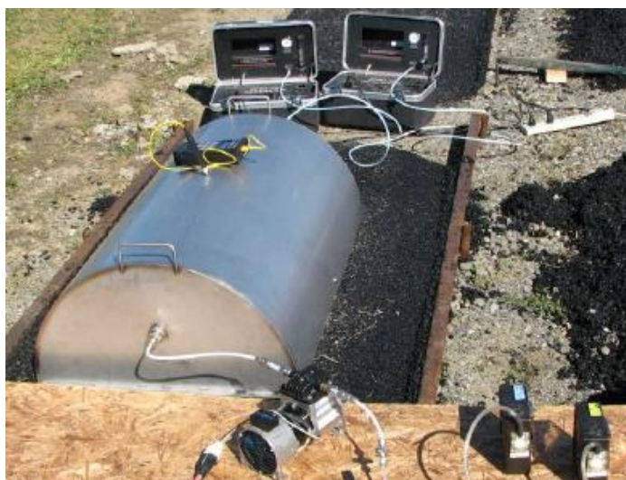
Figure 6.2: University of California portable flux chamber during field sampling
