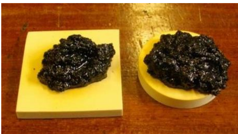
Figure 9.9: CRM binder with 25% crumb rubber prepared on silicone rubber mould for DSR testing
