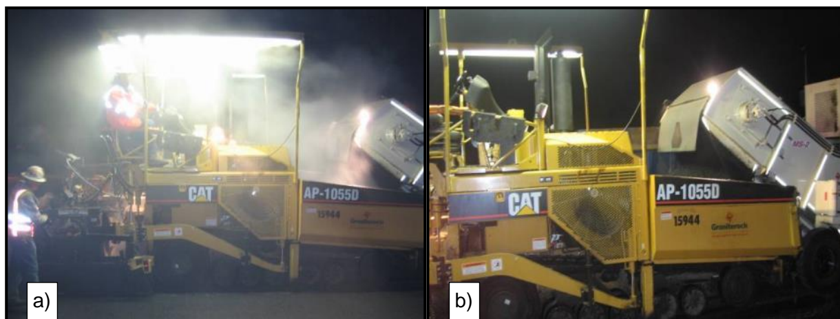
Figure 8.1: a) hot mixed CRM binder asphalt, b) warm mixed CRM binder asphalt
