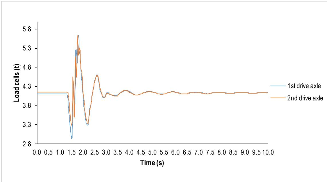
Figure 6.52: Reference system (linear displacement) data trace from RFSA test – 2 shock absorbers removed
