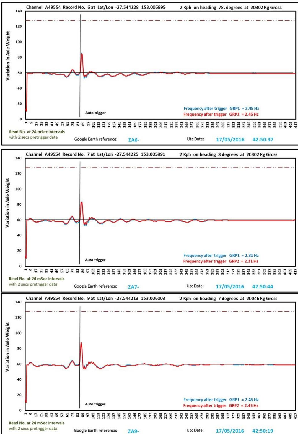
These results showed that neither the damping nor frequency of the suspension could be accurately measured when conducting a 'pipe test' at a speed of 20 km/h. This is because when travelling at a speed of 20 km/h the impulse provided by the pipe was insufficient to excite the suspension with sufficient magnitude. At this point in the test program, it was decided to continue evaluating the method, but at a lower speed (3–5 km/h).
