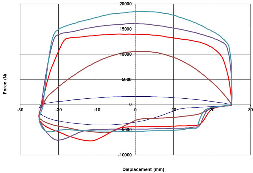
Figure 3.4: Force vs displacement test results for a medium-duty shock absorber
