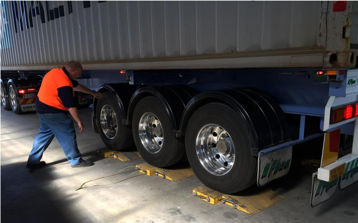
The vehicle should be travelling at 5 km/h when it falls off the step, which is not possible from a standing start, nor is it possible to have a 'run-up' as the disturbance created as the wheels mount the steps invalidates the response. For these reasons the VSB11 ramps are not considered to be suitable excitation method for in-service testing. The variability in the test results (due to small differences in the position of the blocks between tests) confirms this finding.
