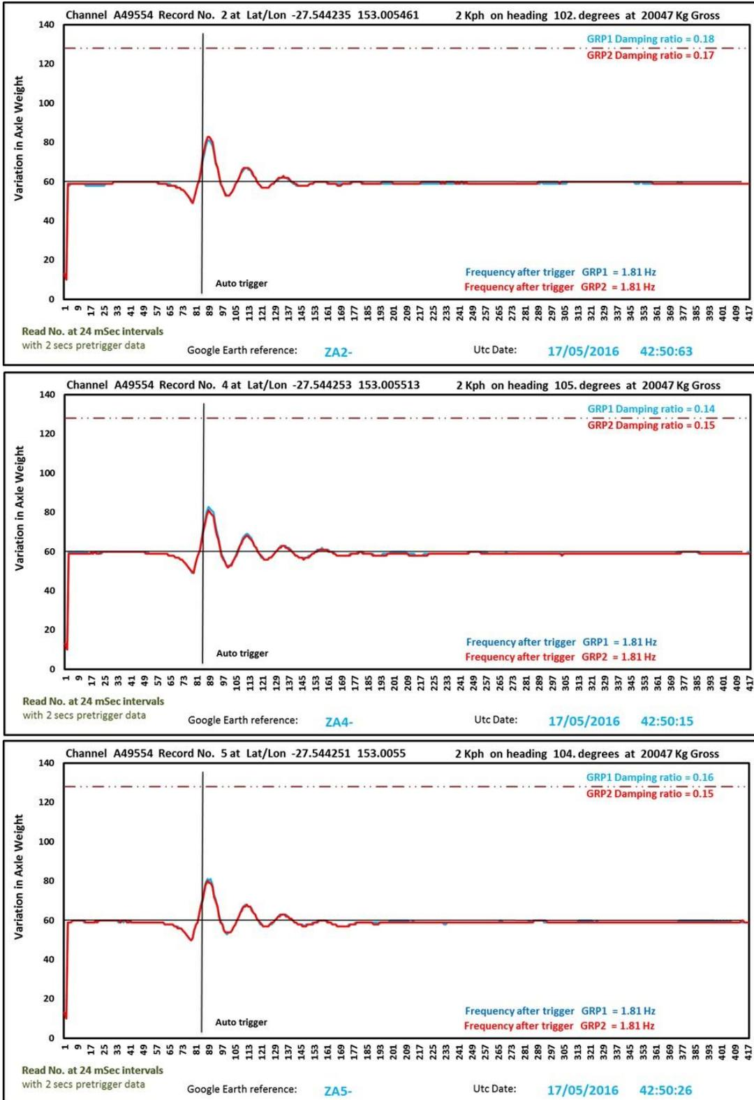
The frequency of each test is identical (1.81 Hz), this is expected as, frequency should not change. The damping ratio varies between left and right sides and between tests. The variation between the left and right is 0.1, varying between tests to be either above or below the other side. The damping ratio varies between 0.14 and 0.18, which is an increase of 28.5%.
