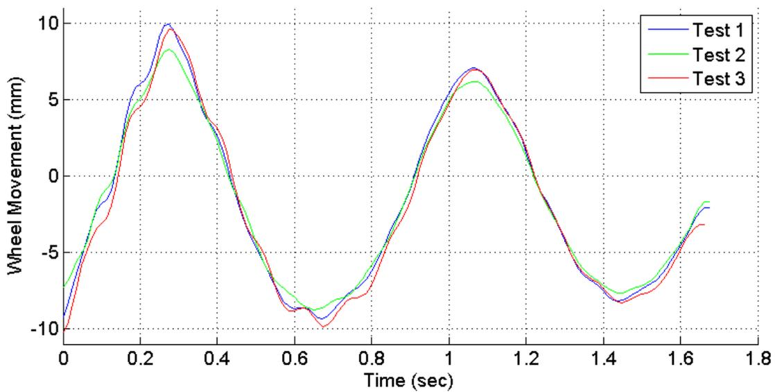
Figure 6.67: Reference system data from VSB11 ramp test method with all shock absorbers removed
