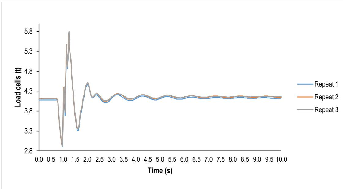
Figure 6.46: Reference system (linear displacement) data trace from RFSA – HD shock absorbers
