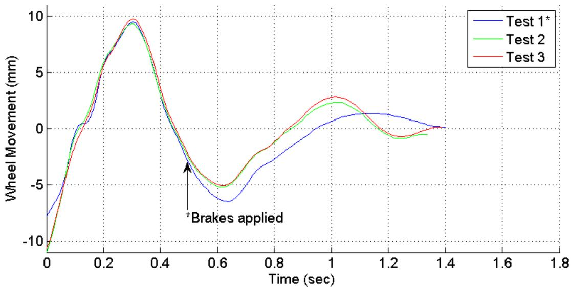
Figure 6.56: Reference system data from DynaSsess test method with all shock absorbers in place
