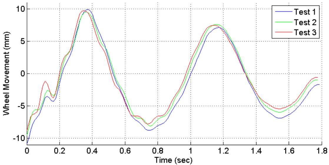
Figure 6.61: Reference system data from DynaSsess test method with all shock absorbers removed
