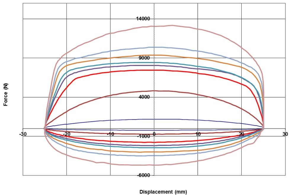
Figure 3.5: Force vs displacement test results for a low-damping shock absorber
