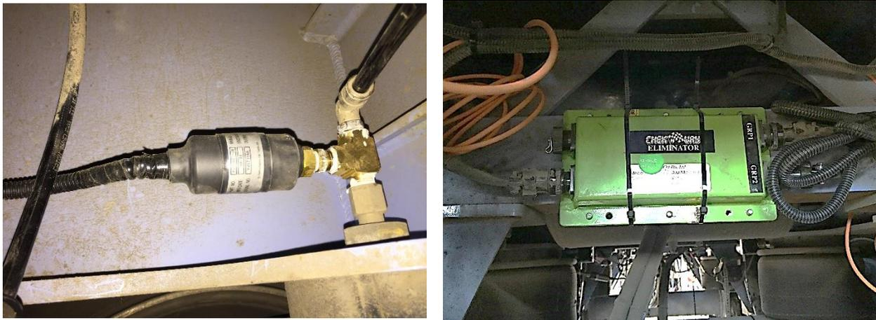
Figure 5.8 shows the reference system fitted to the triaxle semi-trailer. The left photo shows the linear displacement transducer measuring vertical axle displacement and the air pressure transducer. The right photograph shows the accelerometer fitted to the axle and the junction box mounted to the chassis cross-member.
