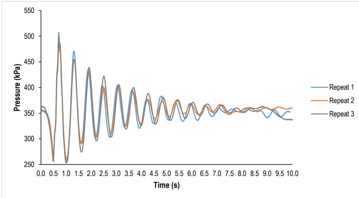
Figure 6.17: Repeatability of pipe tests (no shocks – fully laden)
