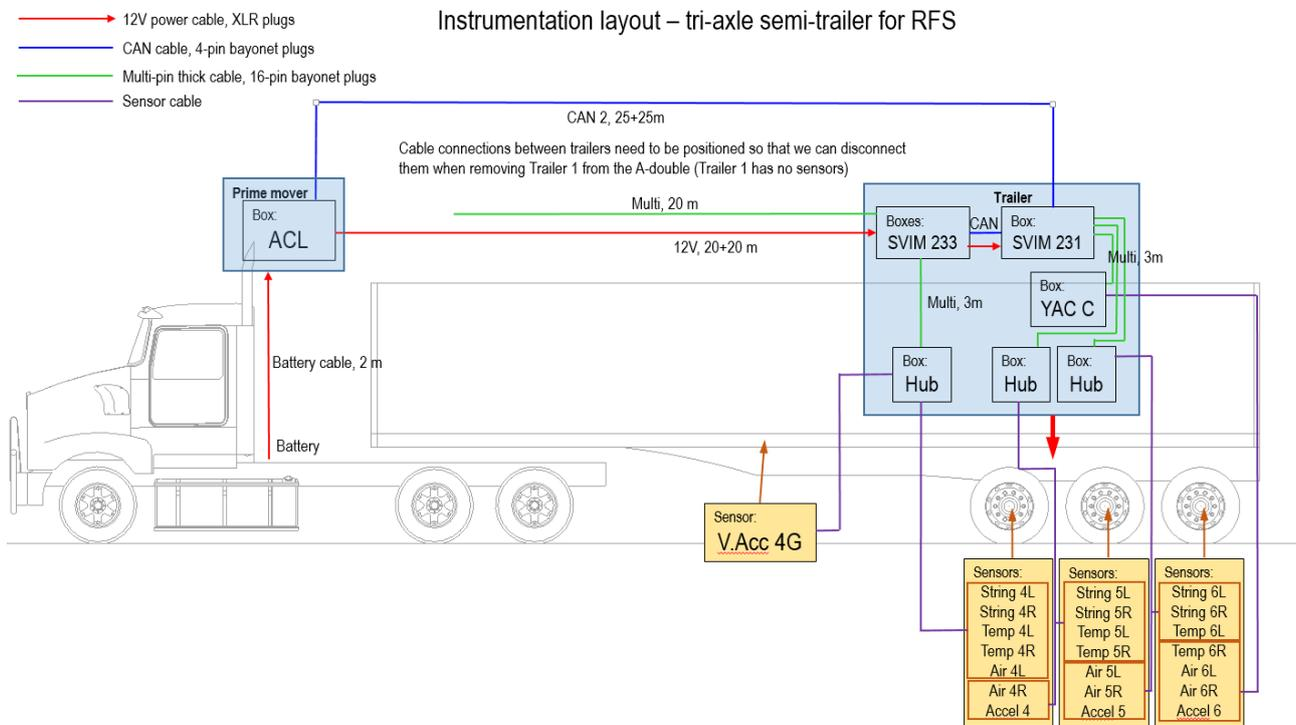
The same instrumentation layout was used for test vehicles 2 and 3, but as these vehicles were fitted with a tandem axle group and single axle, less sensors were required.
