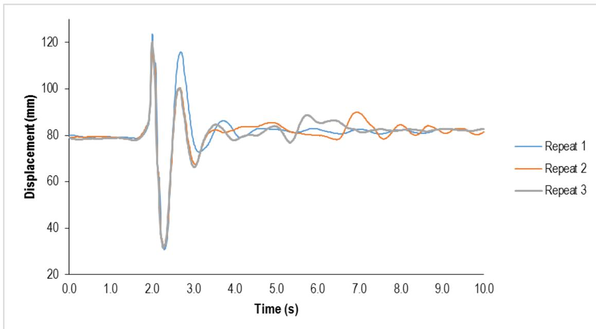
Figure 6.57 shows the data traces for the DynaSsess test with the vehicle with all shock absorbers in place. These results are for the repeat test which was conducted on a flat concrete surface; this test was conducted to replace the earlier test which had been affected by the brakes being applied.
