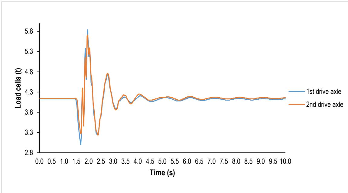
Figure 6.50: Reference system (linear displacement) data trace from RFSA test – 1 shock absorber removed
