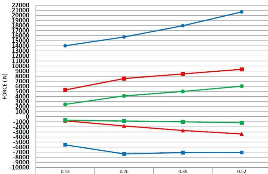
A summary of the peak damping forces for each of the shock absorbers is shown in Table 3.2, Table 3.3 and Table 3.4 for the low, medium and high-damping shock absorbers.
