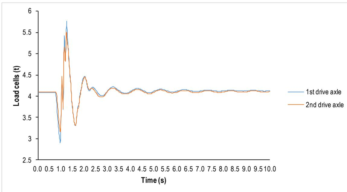
Figure 6.48: Reference system (linear displacement) data trace from RFSA – HD shock absorbers
