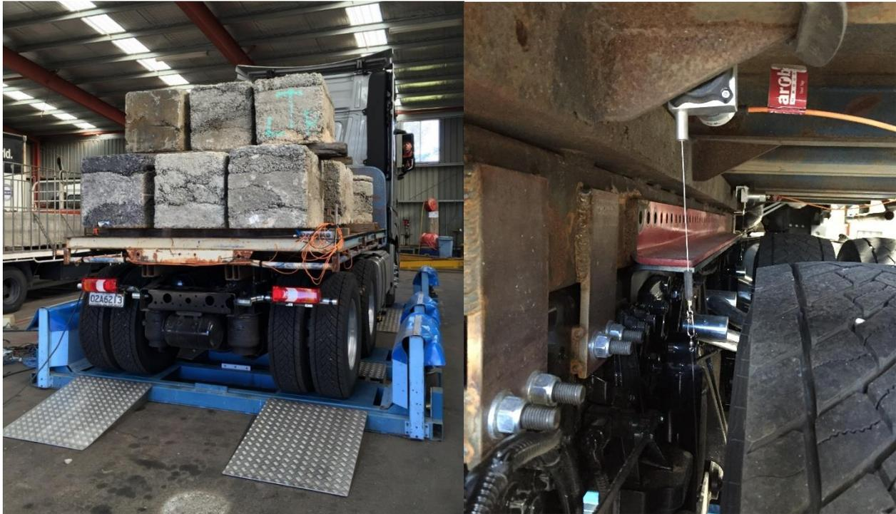
Figure 5.10 shows test system 3 fitted to the rear axle of the 4x2 rigid truck. Test system 3 comprises three main components – the measurement device fitted to the hub and shown in the left photograph, the excitation device (the ramps) shown in the right photograph, and the analysis software (not shown).
