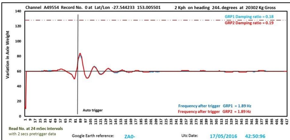
The processed data is 'zeroed' at a baseline value of 60 units. Therefore, this value represents no (zero) vertical displacement between the axle and the body. It should be noted that air pressure transducers measure a voltage linearly proportional to the pressure, not displacement so this is not a direct measure of displacement. The damping ratio can be calculated by using subsequent peak values, as would be done by measuring the oscillation in vertical displacement, as per VSB11.
