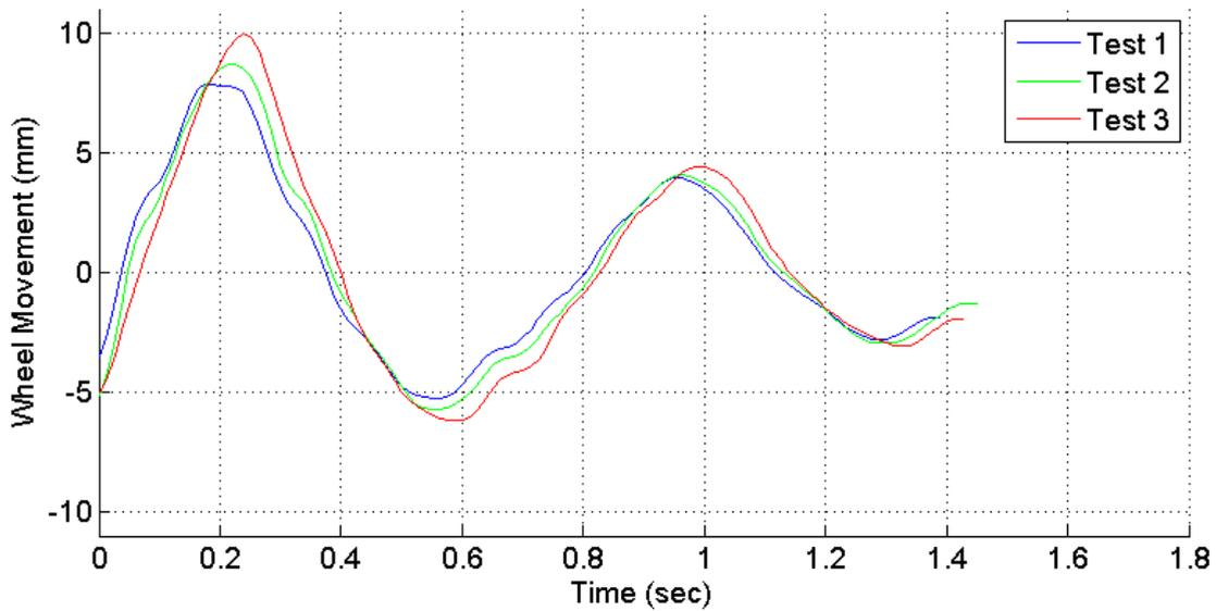
Figure 6.65: Reference system data from VSB11 ramp test method with 1 shock absorber removed
