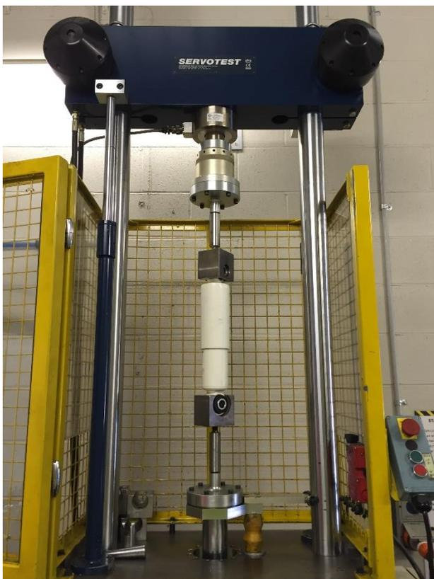
Each shock absorber was cycled through a warm-up procedure and a range of test speeds to measure the damping force prior to be used in the RFS field tests, as shown in Figure 3.2.
