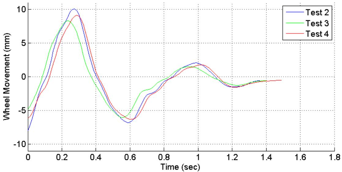
Figure 6.63: Reference system data from VSB11 ramp test method with all shock absorbers in place
