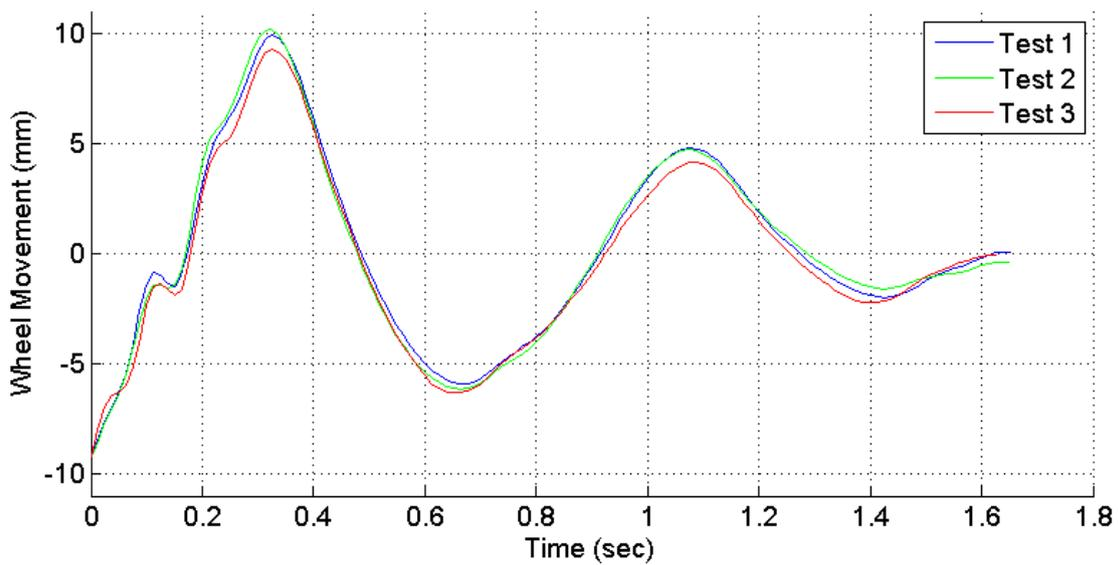
Figure 6.59: Reference system data from DynaSsess test method with 1 shock absorber removed
