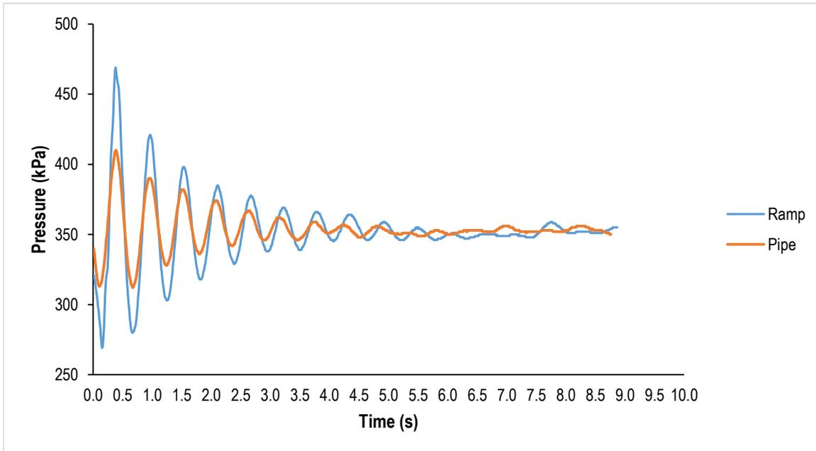
Figure 6.19: Comparison of pipe and ramp tests using LDTs (LOW shocks – fully laden)
