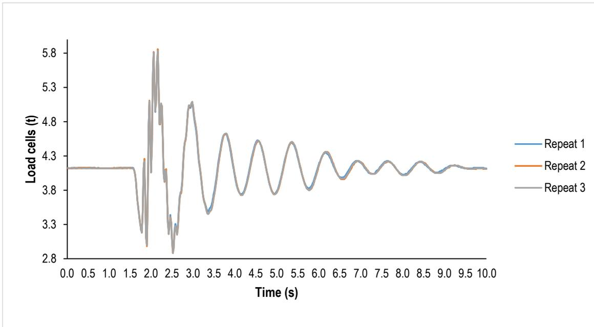
Figure 6.54: Reference system (linear displacement) data trace from RFSA test – all shock absorbers removed
