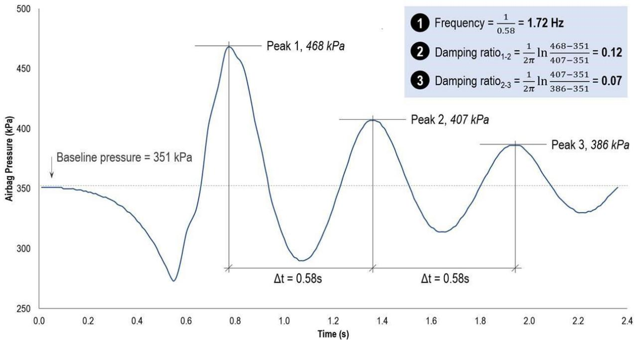
The other important step in analysing the data is to select the baseline value. It can be difficult to determine the true baseline value, particularly if the axles in the suspension group settle at different positions following the test. Figure 7.4 shows the variation in damping when using different baseline values. This example based on data from test program 1 shows a damping ratio of 20% or 24% depending on which value is used.
