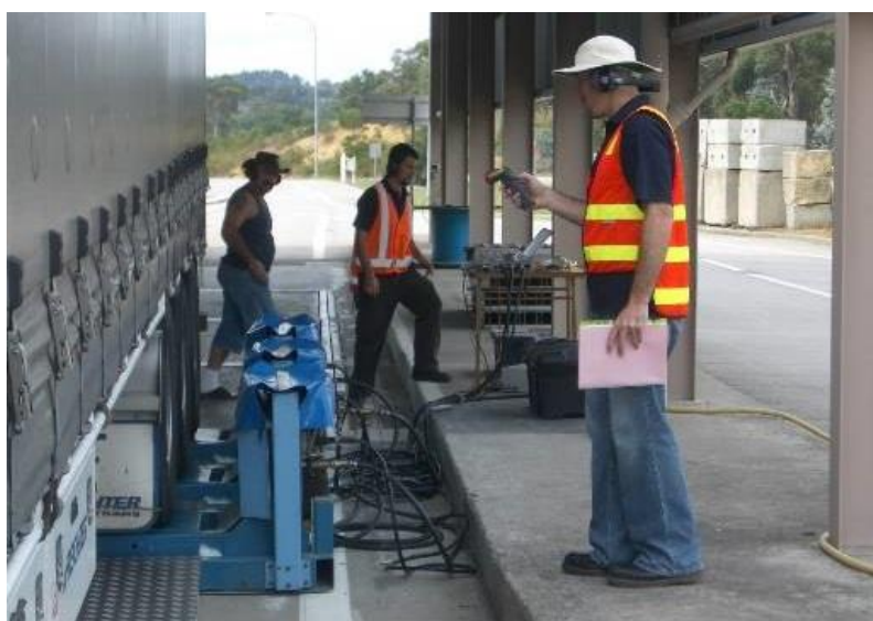
Figure 6.7: RFS testing on site using ARRB RFS analyser
