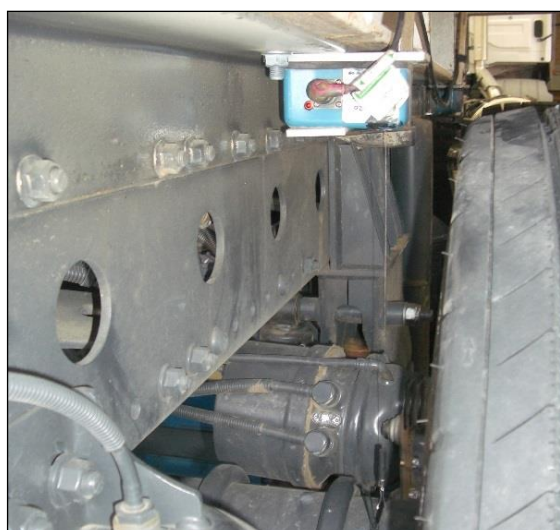
Figure 6.3: Linear displacement transducer fitted to axle
