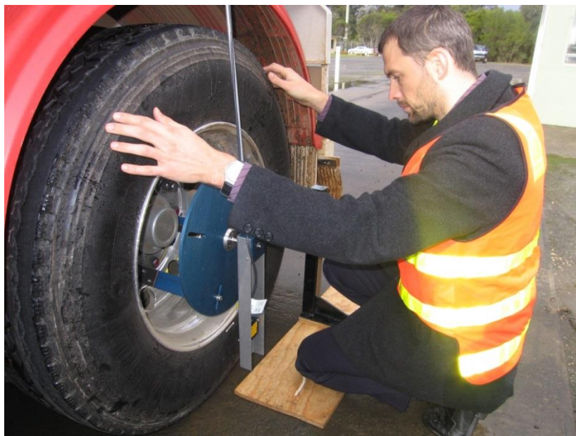
Figure 4.3: Laser mounted hub for measuring dynamic wheel loads
