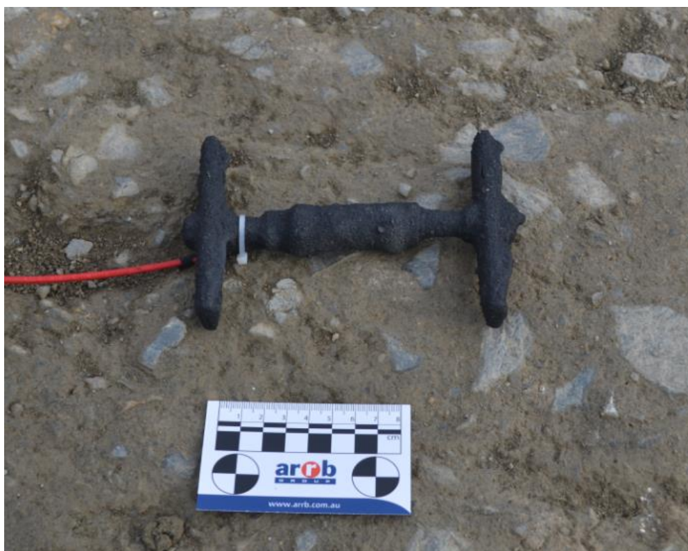
Figure 3.1: CTL Group strain gauge, with protective tack coating applied
