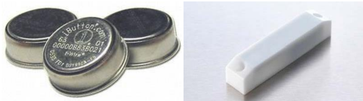
Figure 2.1: Thermochron iButtons (left), Identec i-Q350 tag (right)
