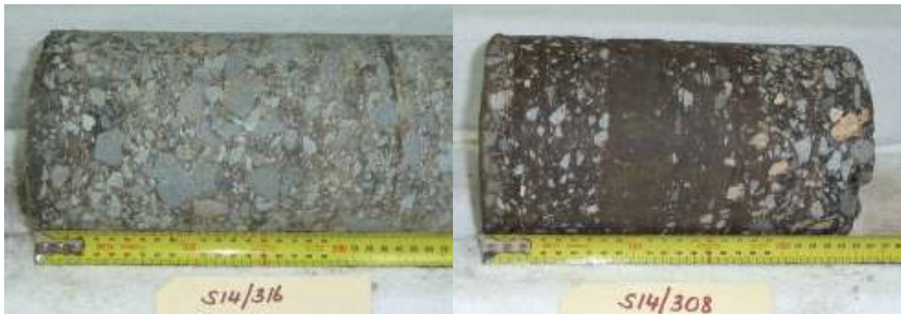
Figure 9.5: I-FBS core specimens from Mt Lindesay Highway (25B) (left) and Bruce Highway (10N) (right)
