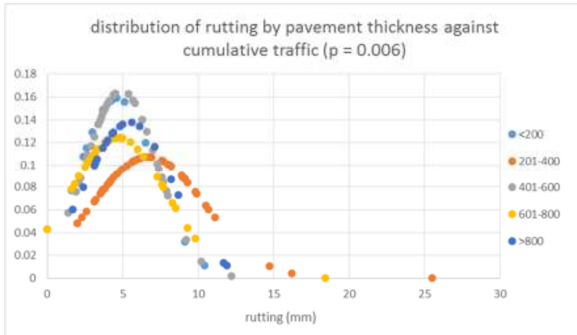
Figure C 4: Distribution of rutting grouped by pavement thickness bins against cumulative traffic
