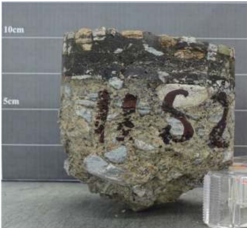
Figure 9.3: PM-CMB core specimen from Bruce Highway (10M) chainage 118 850
