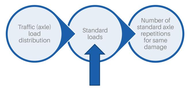
Based on the peak surface deflection being the same as under a standard axle
