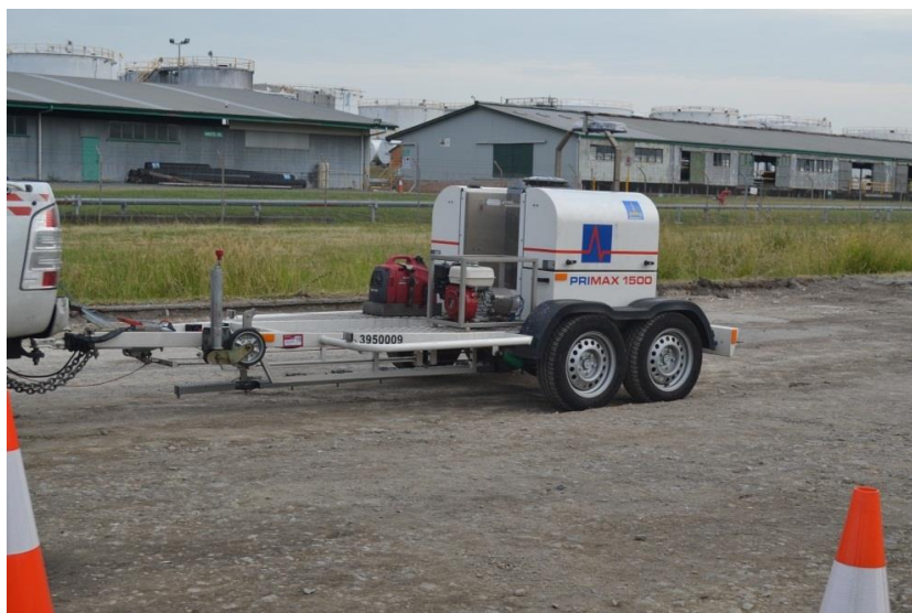
Figure 7.20: Falling weight deflectometer testing on the profiled surface
