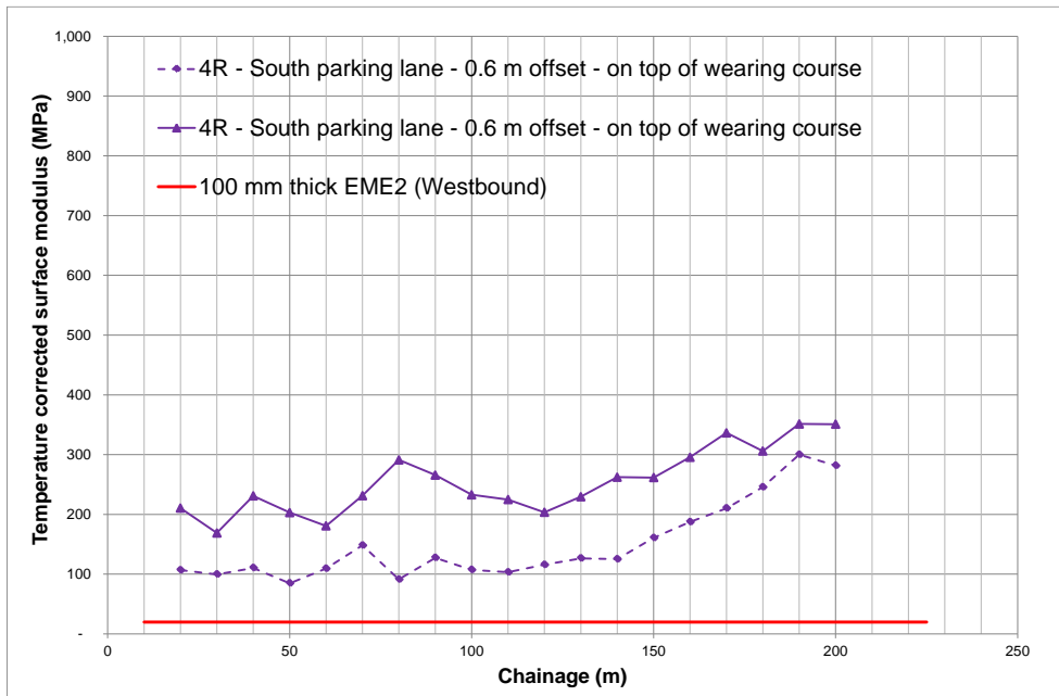
Figure 7.28: Temperature-corrected surface modulus, Cullen Avenue West, south parking lane (4R)
