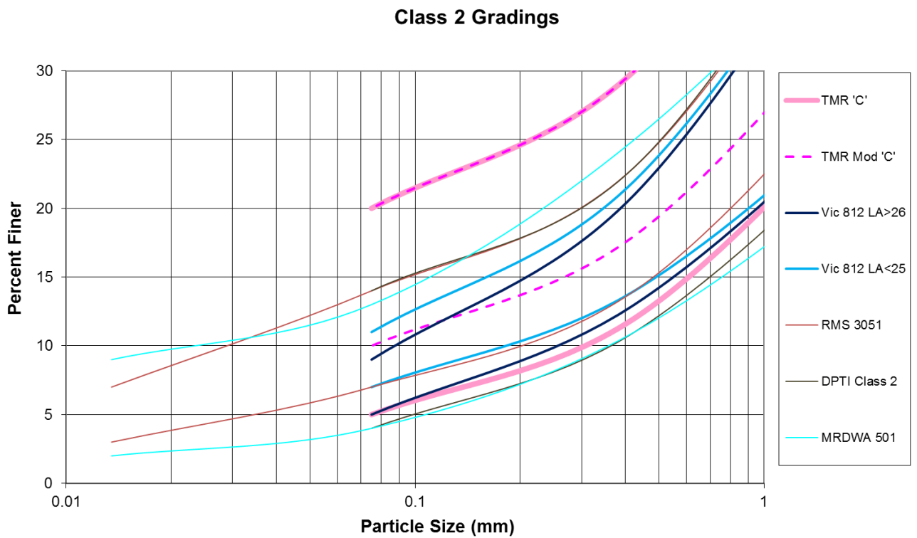
Figure 2.3: TMR C grading comparisons - zoomed in to < 1 mm
