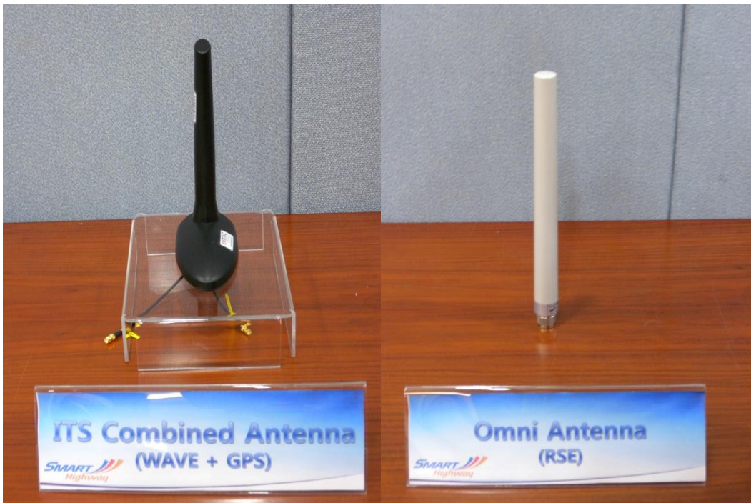
Figure A 7: Combined antenna for WAVE and GPS (left), roadside omni-directional antenna (right)
