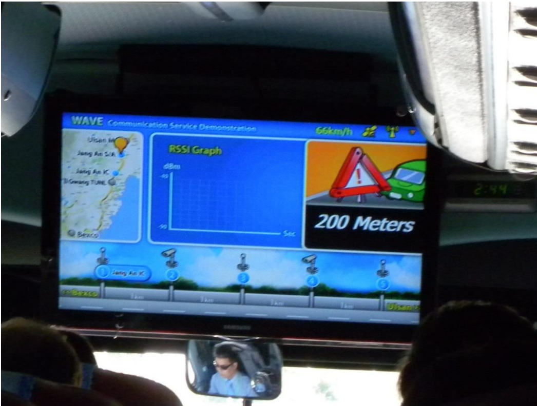
Figure A 8: In-vehicle display developed for demonstration using LCD TV
