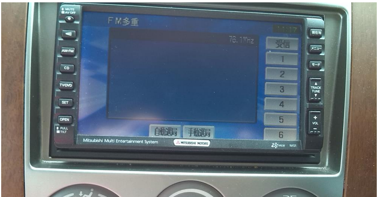
Figure 3.5: Traffic conditions (text feed) via FM, selection of stations (multiple traffic FM stations available in Japan)
