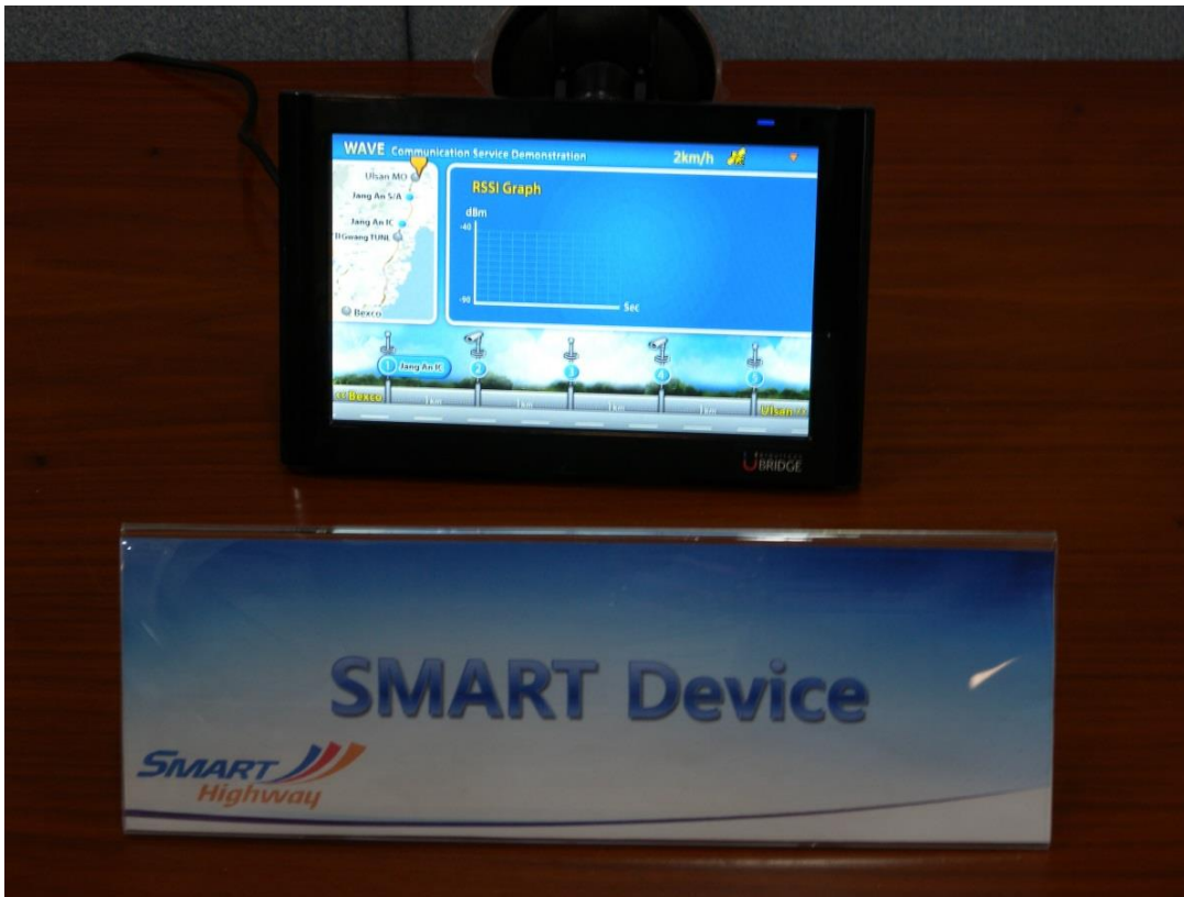
Figure A 6: In-vehicle display, which can be a generic LED or LCD screen connected to the OBU
