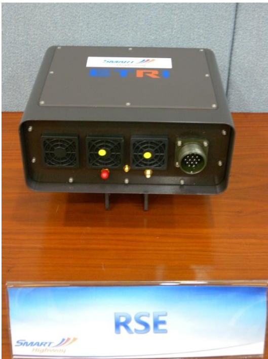
Figure A 9: Programmable roadside device for WAVE (V2I) applications
