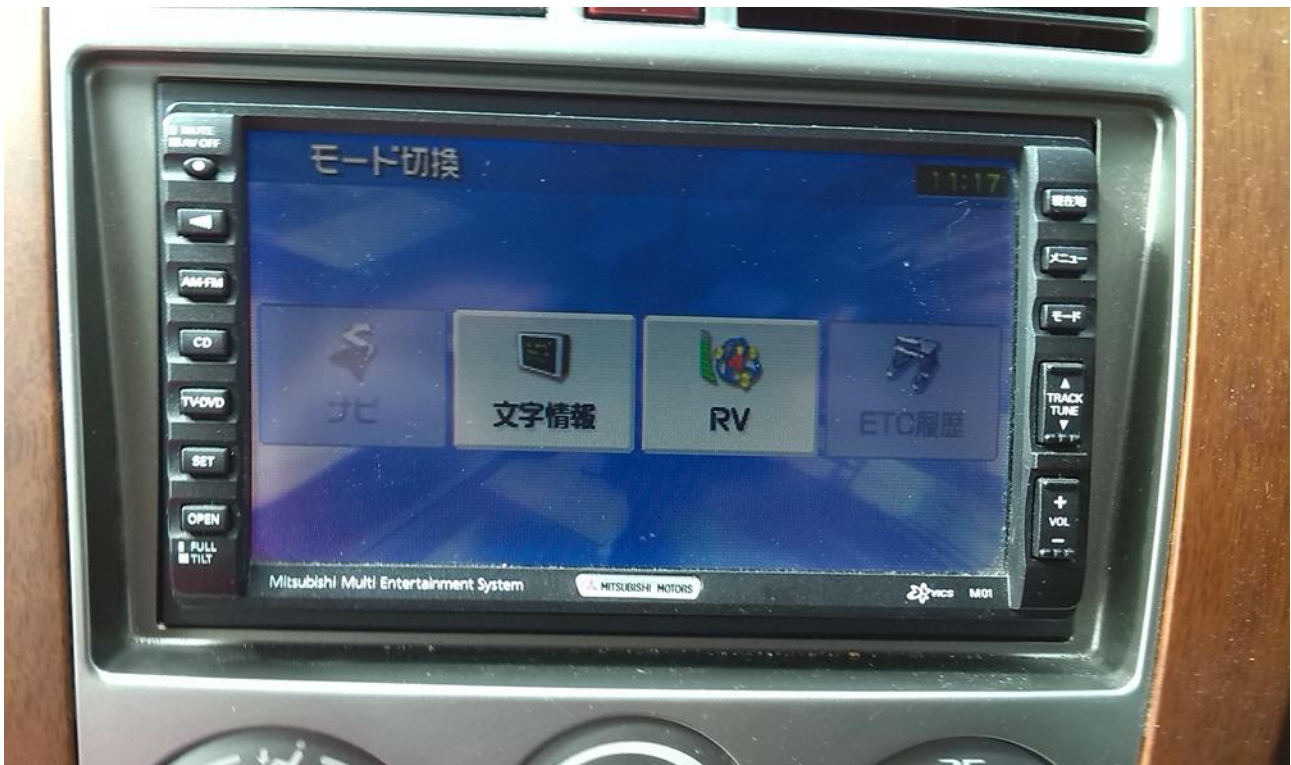
Figure 3.4: VICS in-vehicle unit, icons from left to right are (route guidance, traffic conditions (text feed), compass and road tolling history)
