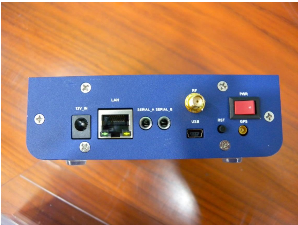
Figure A 11: Back panel of on-board unit (equipment), noting serial, USB and LAN compatibility for connecting a range of equipment for potential applications
